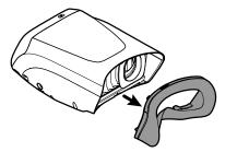
5. If the face cup is attached to the Anterior Imaging Spacer, remove the Anterior Imaging Spacer.
