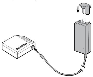
2. Connect the charger's output cord to the charge plug on the battery.
