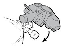
After completing an examination, flip up the BIO module to disengage the magnets, disconnect power, and turn off the light.
