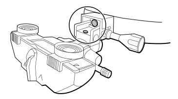
To perform an examination, flip down the BIO module into operating position in front of your face. The magnets engage, connect the LED light source to the power source, and turn on the light.
