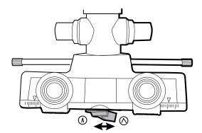
In practice, it's best to use the narrow setting first to obtain the fundus view. Then you can adjust for synchronized convergence and parallax by gradually moving the control as far as possible toward the wide setting without inducing a change in the image brightness or stability.
