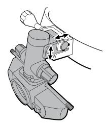
5. Tighten the locking nut to secure the module in place
