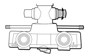
Similarly, the control that selects between small, medium, and large apertures and the diffuser is located on the left side of the control arm when the instrument is on your head.
