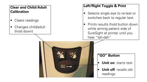
The instrument will turn off when unused for 1 minute. Any button pressed on the SureSight will bring up results.
