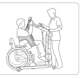
4. Raise the sling bar to the lowest height necessary to perform the transfer.  $\Delta$  Make sure that the lifting motion is not so high that
