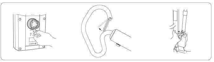
**Electrical emergency lowering/raising** Use a narrow object to push the buttons inside the labelled holes on the control box.
