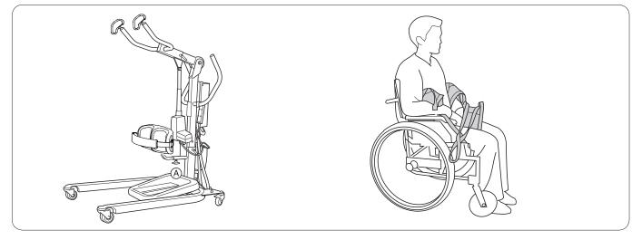
1. Disassemble the lower leg support: Unscrew screw A. Pull out the lower leg support. Remove the foot rest: Grab the front edge of the frame. Fold it up and lift it off the base. 2. Apply suitable sling according to the sling's instruction guide. Above Liko HygieneSling mod. 40 is applied.
