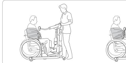
1. Place the ComfortVest around the patient according to the vest's instruction guide. Place Sabina sit-to-stand lift in front of the patient. Adjust the width of the base. Place the feet in the middle of the foot rest with the lower legs parallel to the lower-leg support. Adjust the height and depth of the lower-leg support as needed for comfortable support below the kneecap.
