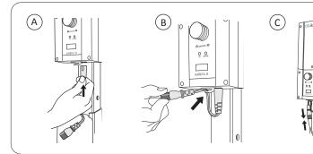
6. A) Connect the charger cable to the socket under the control box.B) Attach the connector cable to the strain relief system.C) Plug the charger cable into the connector cable.
