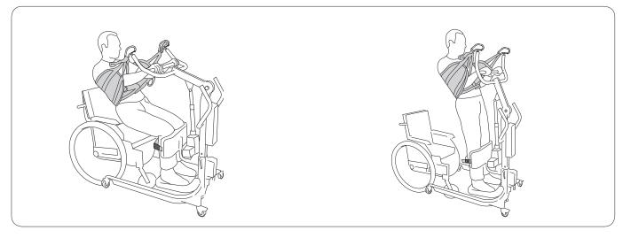
3. Raise the sling bar about 10–20 cm (4-8 in). The patient grabs the sling bar. Continue the lifting procedure. If the patient leans backwards, the raising will be made easier, preventing the vest from sliding up. The height to which the lift should proceed varies from person to person.
