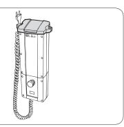
7. Install the holder for the charging cable: Hook it on the front edge of the battery and push down on the back until you hear a clicking sound.
