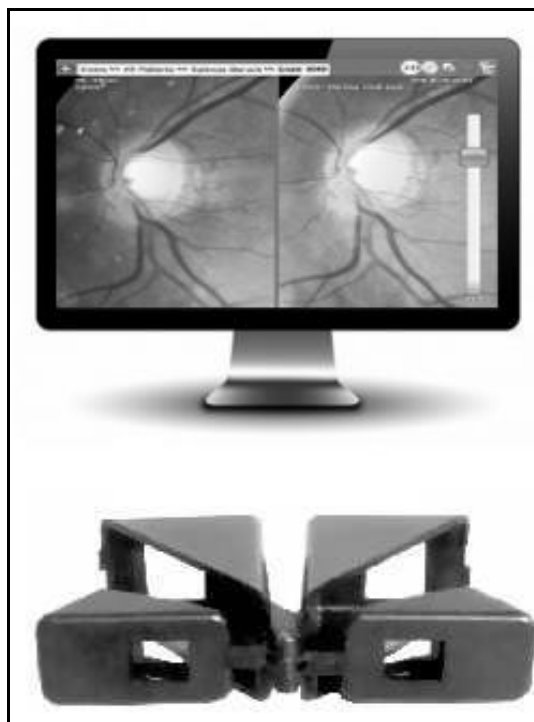
Figure 24 - To perceive the 3D vision of the optic disk, the images must be watched with a couple of prismatic goggles that let each eye see only one of the two images. The photo shows an example of such goggles. “Crossed-eye” format is also supported.
