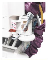
2. Route the power cord underneath the foot board and frame on the left-foot corner of the bed and attach the second magnet to the frame.
