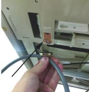
3. Attach the third magnet underneath the intermediate frame on the patient left-hand side of the bed.
