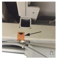
5. Attach the fifth magnet along the intermediate frame near the power drive.
