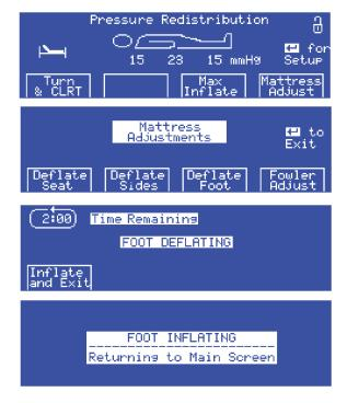
After the foot section has been deflated, the **Deflated Foot** indicator shows on the Pressure Redistribution screen. To inflate the foot section, do as follows:
