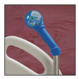
3. Press the green **Transport** control (1) to lower the bed to the transport position (the power drive wheels on the ground). When the bed reaches the Transport position, you will hear a single beep, and the amber **Transport** indicator on the transport pod will turn green.
