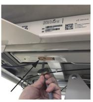
4. Attach the fourth magnet along the intermediate frame near the HiLo drive.
