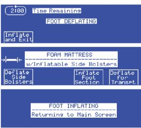
The **Foot Inflating** screen shows, the foot section inflates, and then the **Foam Mattress** screen shows.
