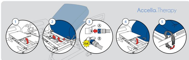
8. Connect the plug to the bed connector (it clicks into place).
